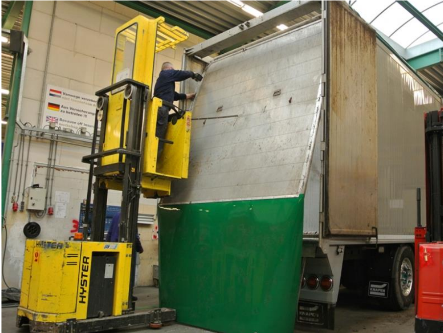
Picture Knapen: Moving headboard undergoing maintenance
