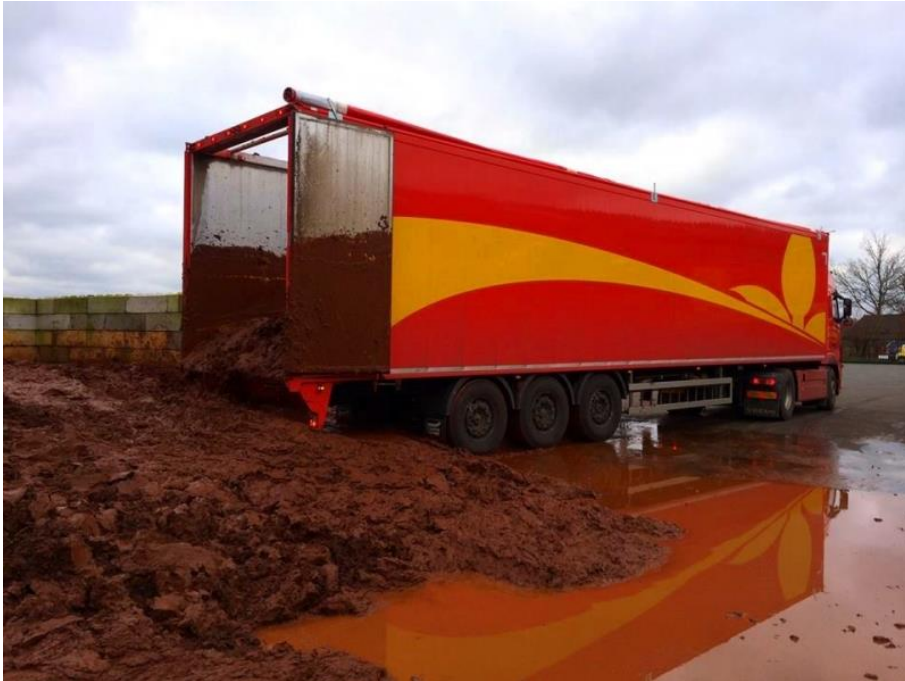
Picture: More liquid loads will put pressure on the doors. Stand clear of the fan shaped danger zone
