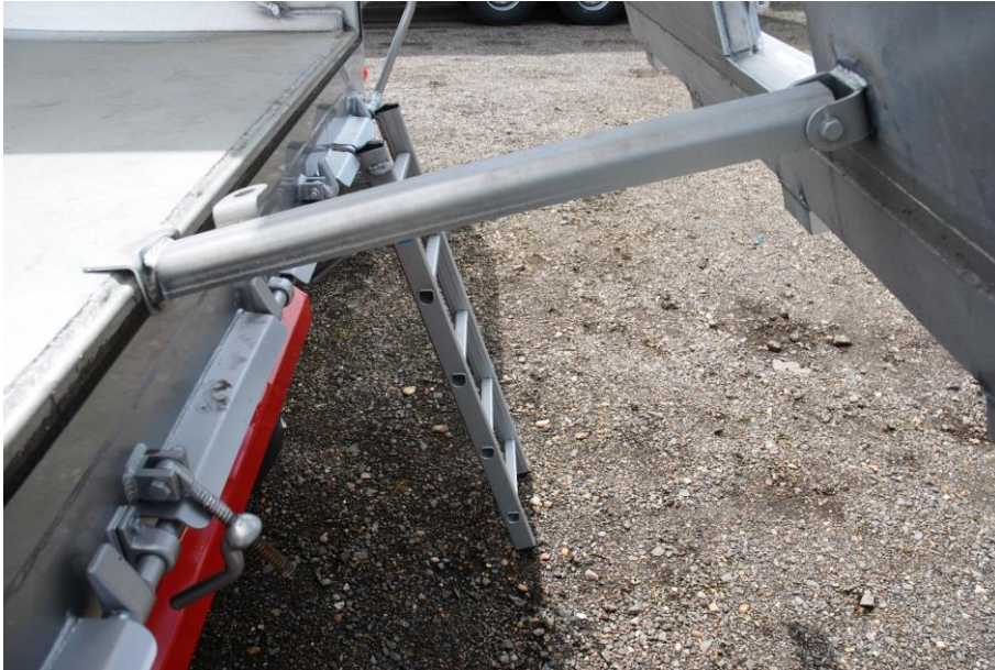
Picture: Rear door safety prop in place, rear door ladder attached with hooks over locking bar
