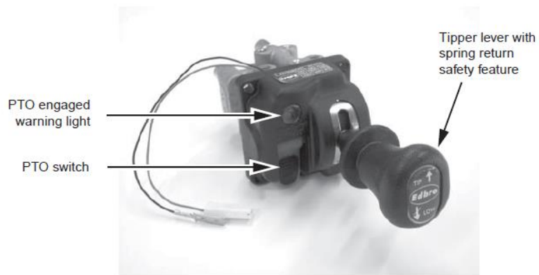
Fig. a. Combined PTO & tipper air controls
