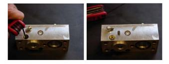
When reassembling please make sure that the seal rings are still present. Further prevent pollution. Tighten the 5 M8 bolts with a torque of 30 Nm. After this the treaded rod or distance ring has to be mounted. (If necessary one can find the directions for adjusting the threaded rod in the operation manual, these also can be found on <a href="https://www.cargofloor.nl/downloads">www.cargofloor.nl/downloads</a>.)
