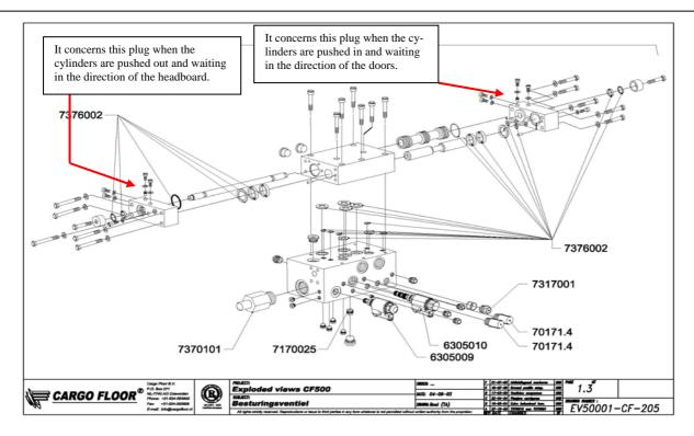
To fix this malfunction one has to demount the threaded rod with the distance ring, or demount the distance ring at the back side.
