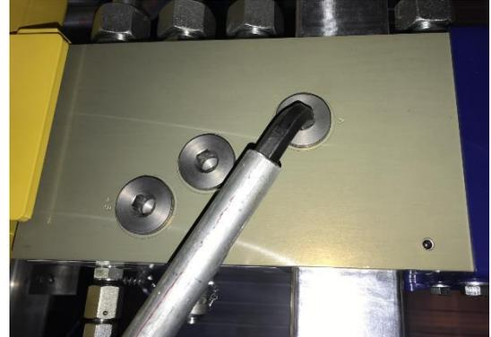
The replacements need a spanner 24 to tighten them. If available, a gear spanner 24 mm (ratchet spanner, gear wrench) does the best job.
