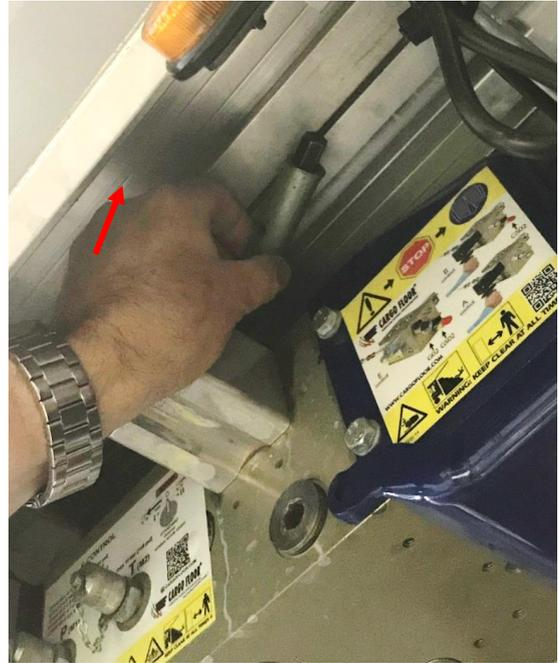
Tighten the plug as tight as possible.
