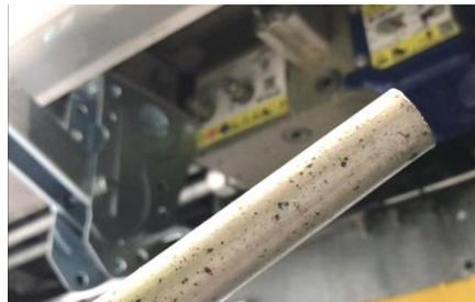
Shorten the short stem of the Allen key (as short as possible) and keep in mind that it still has to go into the hexagon socket of the plug (which is 11 mm deep). Shortening this stem will result in more room for your hand to be able to apply enough force to pull. The plug should be tightened with about 140 Nm or higher.
