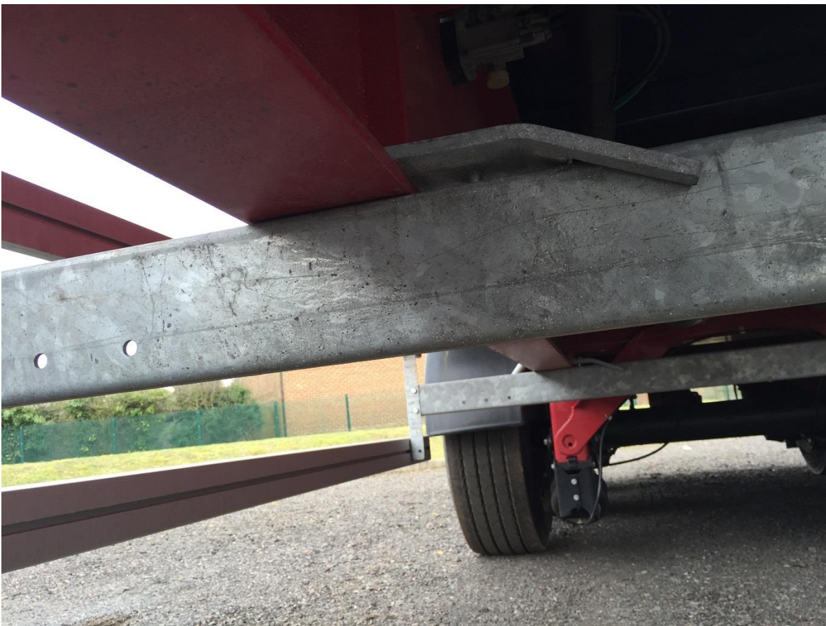
Clamps to bottom rail of the chassis I beam with galvanised clamping brackets.
