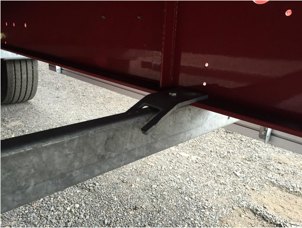
Simple bolt on clamping bracket to fit to trailer bottom flange.
