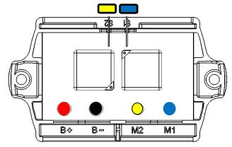
10698 Mechanical Motor Reversing Relay (Rear View)
