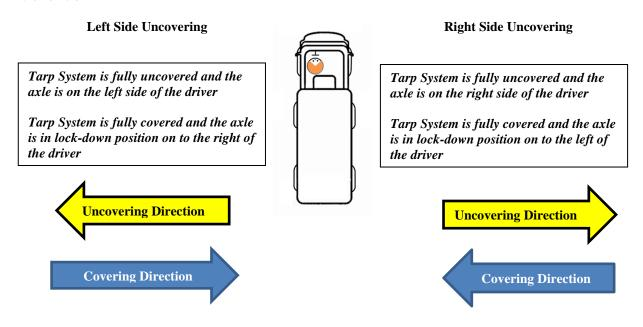
For Front to Back, flip style tarp systems, follow the orientation of the Right Side Opening Side to Side Systems
