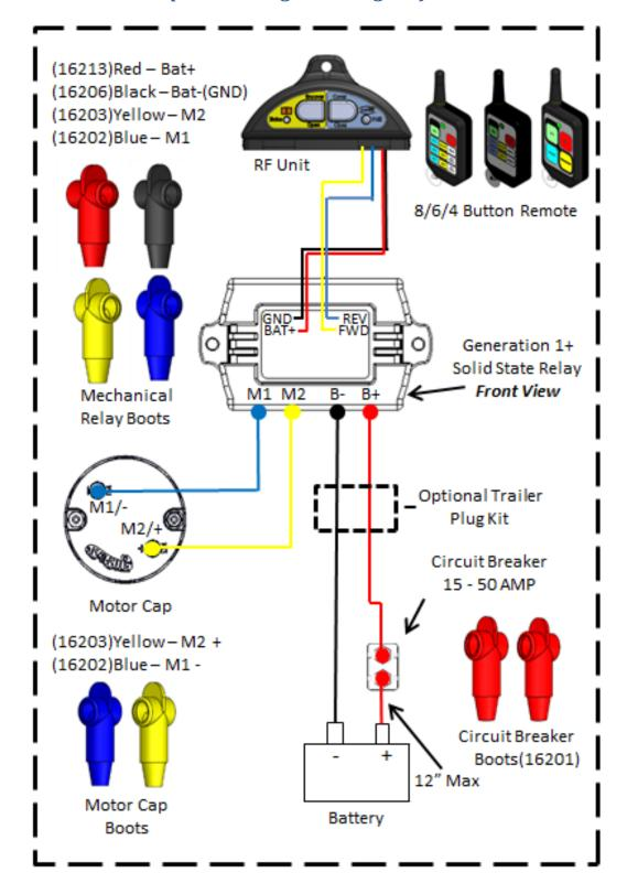
Generation 1+ Rite Touch® Solid State Reversing Relay with RF Switch Tarp Uncovering to the Left of Driver
