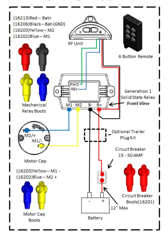
Generation 1+ Rite Touch® Solid State Reversing Relay with RF Switch
