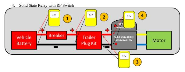
Tip: while moving the probe from left to right, we are checking that voltage is present through all connections. If voltage is lost at any point from 1 to 4 when moving from left to right, it should remain lost for all points to the right of the issue.
