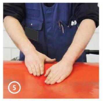
Apply the self-adhesive tape to the cleaned area of sheet to be repaired Firmly press the tape onto the sheet, for several seconds.
