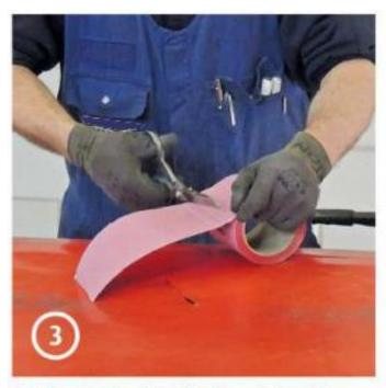
Cut the required length of repair tape, from the roll
