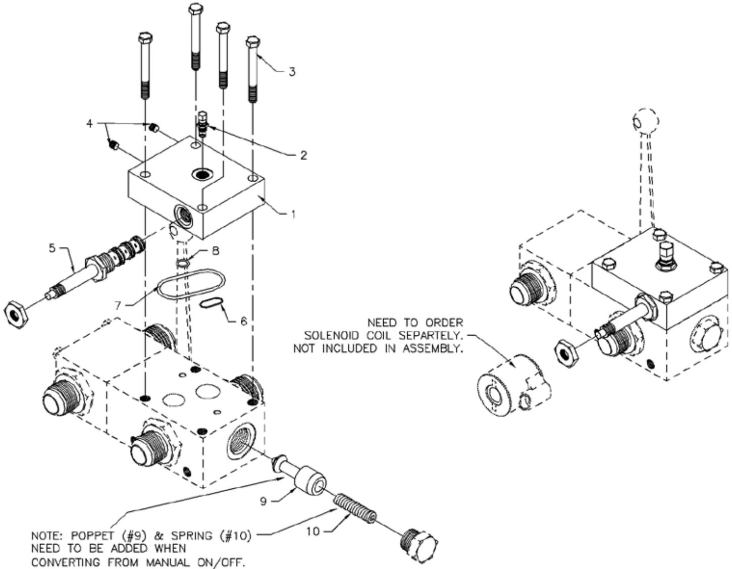
Information For Ordering Solenoid Coil & Connectors: 24 Volt Coil (HF 24 VCD 6353024) – Part #85602000
