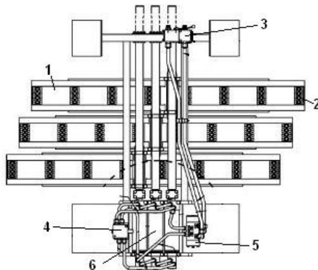
Figure 1.1: KEITH WALKING FLOOR Workhorse drive-unit
