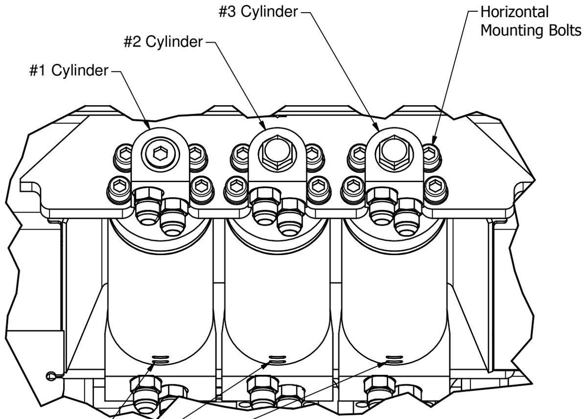
Note wire lock slot width for cylinder model identification.
