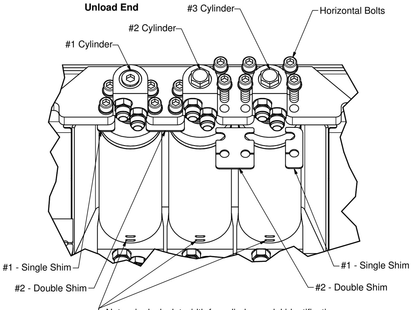
Note wire lock slot width for cylinder model identification.
