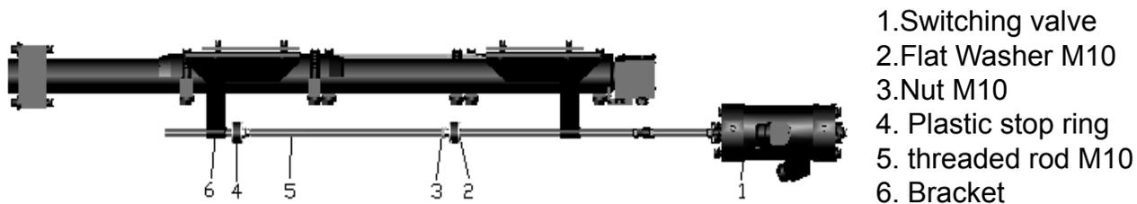
Figure 7.1 : Adjustment of the switching valve
