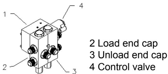
Figure 5.5b: *The Electric Control valve* 1 Pilot valve housing
