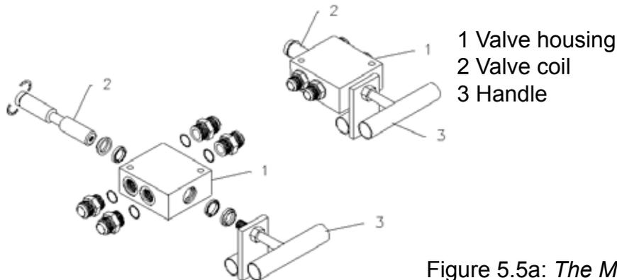
Figure 5.5a: *The Manual Control valve*
