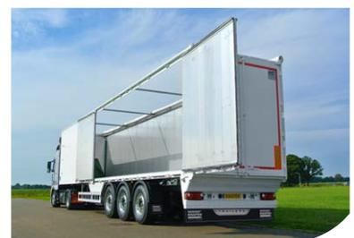
Self-supporting construction with side opening of 6.8m
