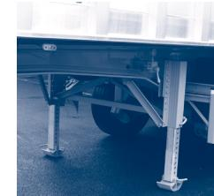
Figure 2.3.1.a. – "Aluminium type" landing leg
