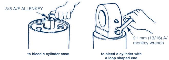
Figure 3.2.a. - Cylinder venting
