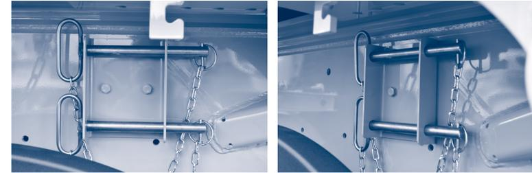
Figure 8.4.2.a. – Position of levers for blocking automatic hinged rear under-run bar
