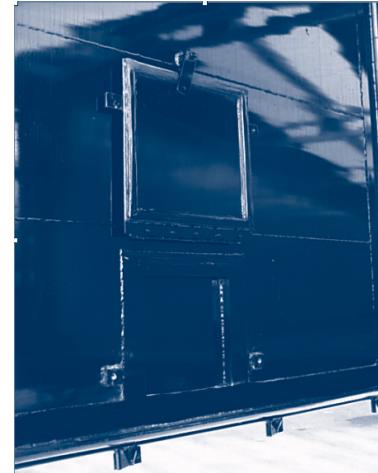
Figure 6.4.1.b. – Grain hatch on leakproof door, plate with seals folded away
