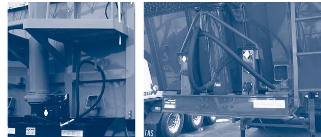
Figure 2.3.2.a. – Hydraulic connection single-line system (left), two-line system (right)
