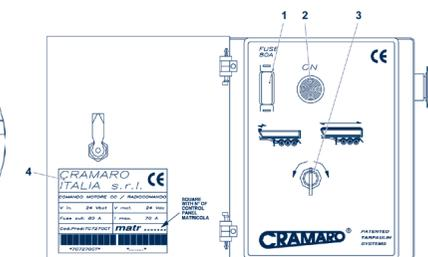
Figure 7.4.2.c. – Operating panel, electrically operated roof sheet, type “Cramaro”
