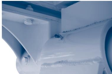
Figure 6.c. – Lubricate tipper turning points
