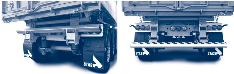
Figure 8.4.1.b. – Automatic hinged rear under-run bar
