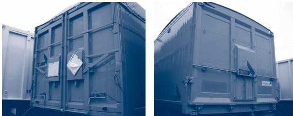
Figure 8.2.1.a. – Different types of grain hatches
