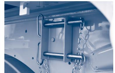
Figure 8.4.2.a. – Position of levers for blocking automatic hinged rear under-run bar
