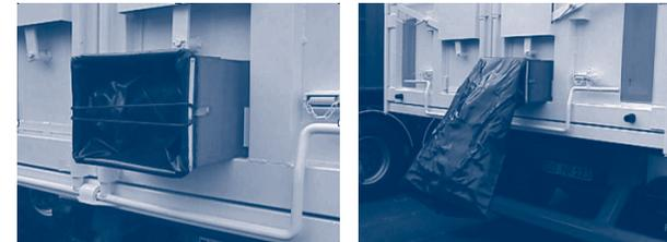
Figure 8.2.1.b. – Door with grain hatch with dust sleeve
