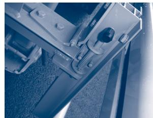
Figure 10.3.b. – Pull out safety pin and folding side guard upwards
