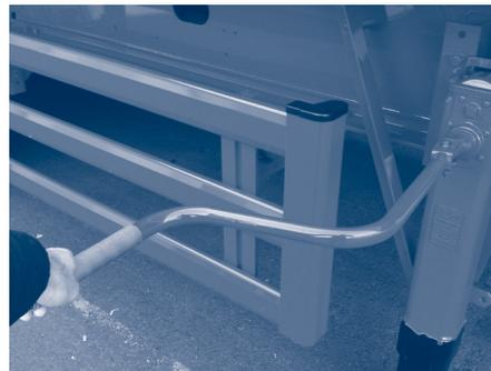
Figure 2.2.1.c. – Landing leg handle "steel type"
