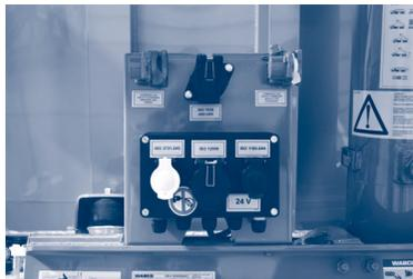
Figure 3.3.a. – Connection braking system
