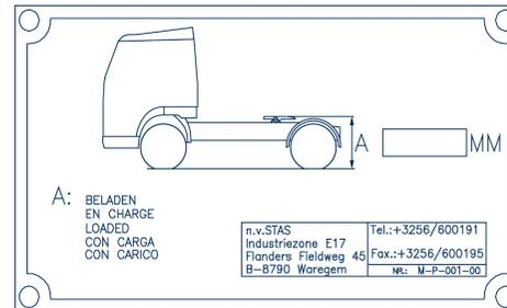
Figure 1.c. – Sticker coupling height for 2-axle lorry
