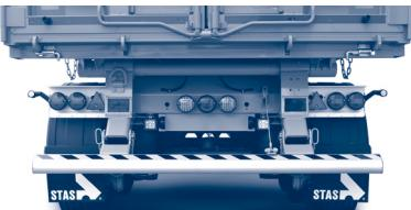
Figure 8.4.1.b. – Automatic hinged rear under-run bar
