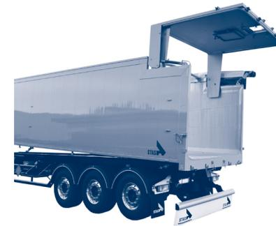
Figure 6.5.1.a. – Tipper with hydraulic top hinged door
