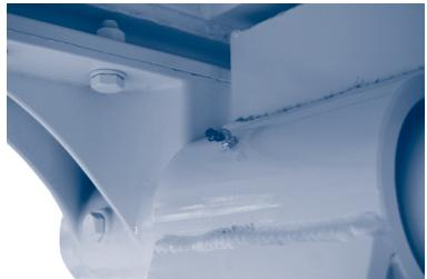
Figure 6.c. – Lubricate tipper turning points
