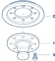
Figure 1.1.a. – Kingpin (1), socket (2) and retaining bolt (3)
