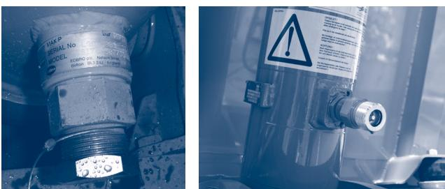
Figure 4.1.a. – Cylinder type plate + maximum cylinder pressure pictogram
