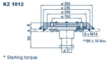
Figure 1.1.b. – Kingpin with aluminium fifth wheel rubbing plate
