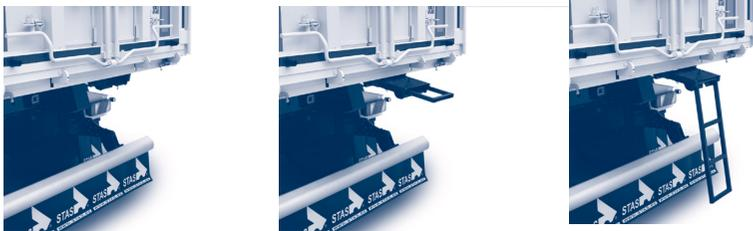
Figure 10.2.a. – Ladder (optional) for access to loading area
