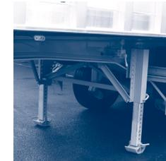
Figure 2.3.1.a. – "Aluminium type" landing leg
