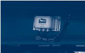
Figure 8.3.a. – Bodyguard (left: main control unit right: proximity switch with detection plate)
