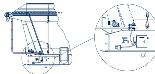
Figure 7.4.2.a. – Electrically operated roof sheet, type “Cramaro”
