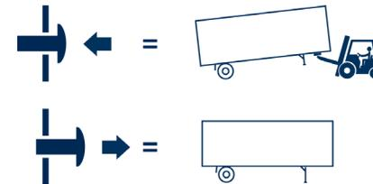
Figure 3.10.b. – Use of the emergency brake
