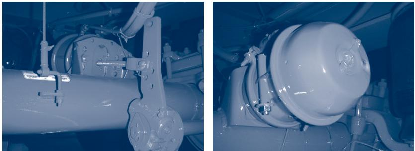
Figure 3.9.a. – spring brake cylinders
