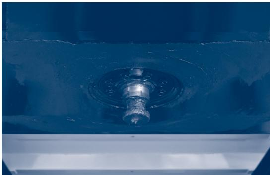
Figure 1.a. – Fifth wheel rubbing plate with kingpin
