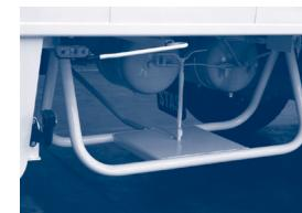
Figure 5.2.a. – Single spare wheel carrier
