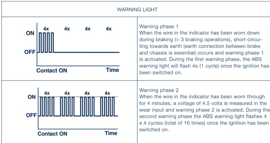
The warning is interrupted when the trailer exceeds a speed of 7 km/hour. In case of system faults, the ABS warning light is permanently activated.
