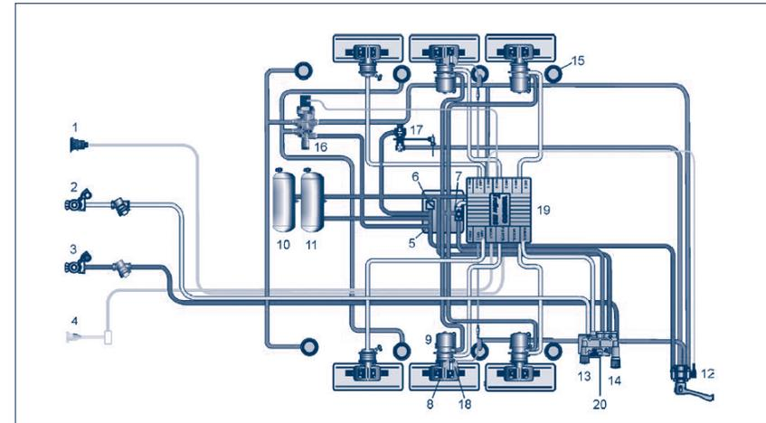
Figure 3.2.1.a. – Example EBS system layout 2S/2M
