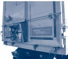
Figure 8.2.1.c. – Operation and locking of the grain hatch, type with rack and pinion
