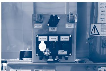
Figure 3.3.a. – Connection braking system
