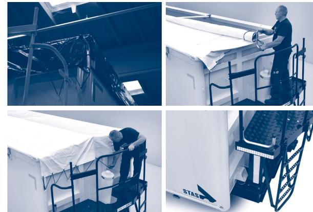
Figure 7.2.1.a. – Attachment winding handle
