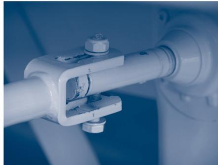
Figure 2.2.1.b. – Landing leg handle "steel type" pulled out
