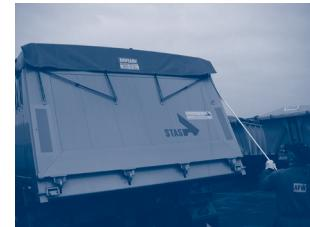
Figure 7.3.2.a. – Fastening pull back cord and loosening of roof sheet
