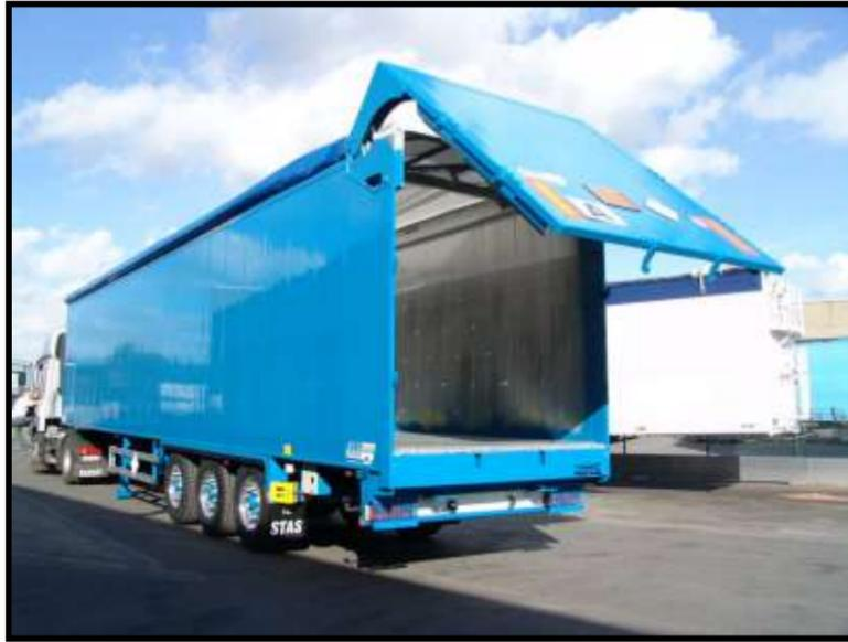
Figure 6.2.a. – Hydraulically operated top swinging door
