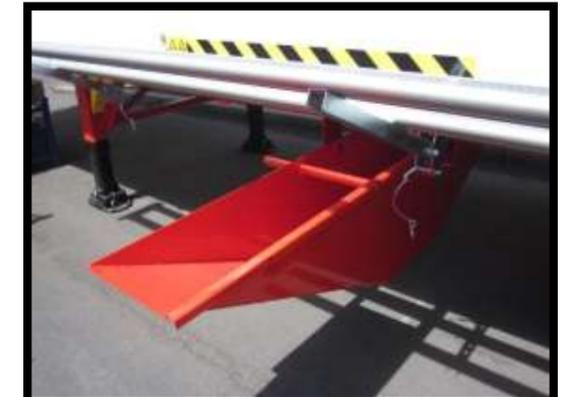
Figure 8.2.d. – Locking pin (left) and sliding of funnel (right)
