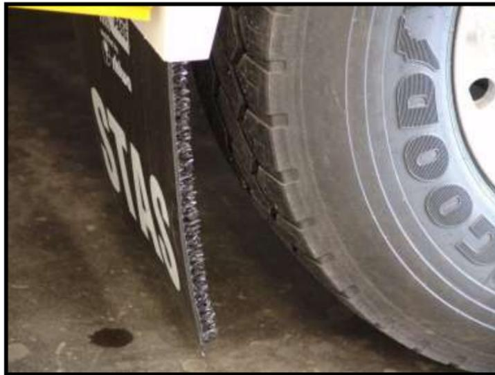
Figure 5.4.b. – Mud flap with spray suppression
