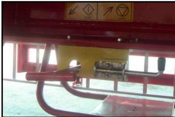
Figure 2.2.4.c. – Unlocked and pulled out mechanical emergency stop lever
