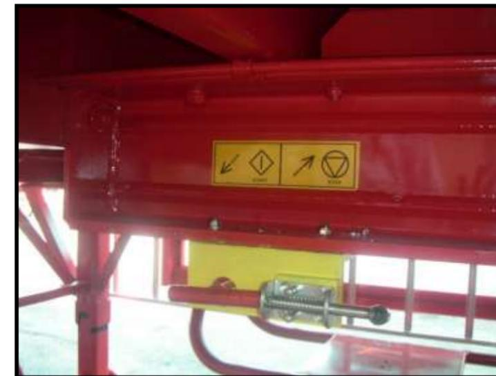
Figure 2.2.4.a. – Mechanical emergency lever in locked position
