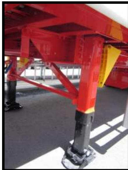
Fig 2.1.a. – Landing legs -“aluminium type
