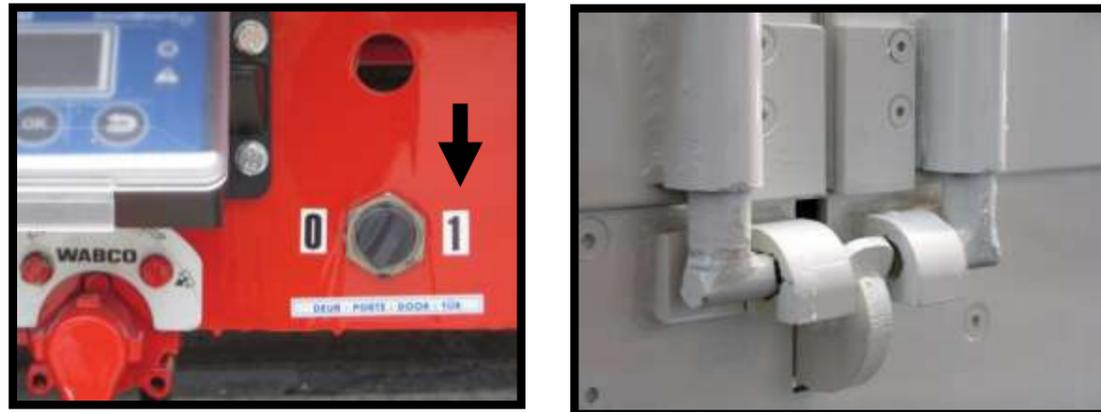
Fig 10.6.a. – “Opening” of door lock (left) and opened door lock (right)
