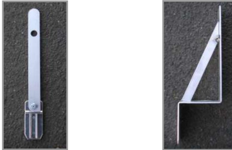
Figure 7.2.b. – Straight (left) and buckled (right) roller stops
