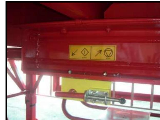
Fig 2.3.3.a. – Mechanical emergency lever in locked position
