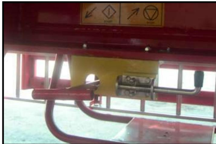
Figure 2.3.3.c. – Unlocked and pulled out mechanical emergency stop lever
