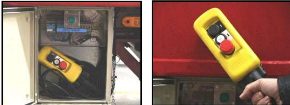
Fig 6.2.b. – Control unit top swinging door (right) with reset button and buzzer in storage area (left)
