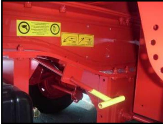
Figure 2.2.4.b. – Selection bar for loading and unloading in loading position
