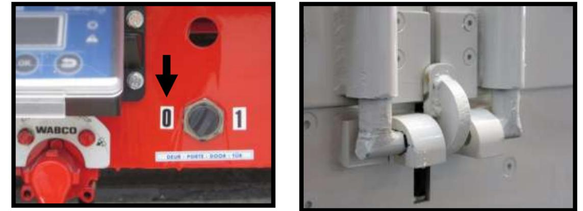
Fig 10.6.b. – “Closing” of door lock (left) and closed door lock (right)
