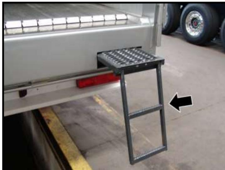
Figure 10.2.a. – Ladder for access to the load space
