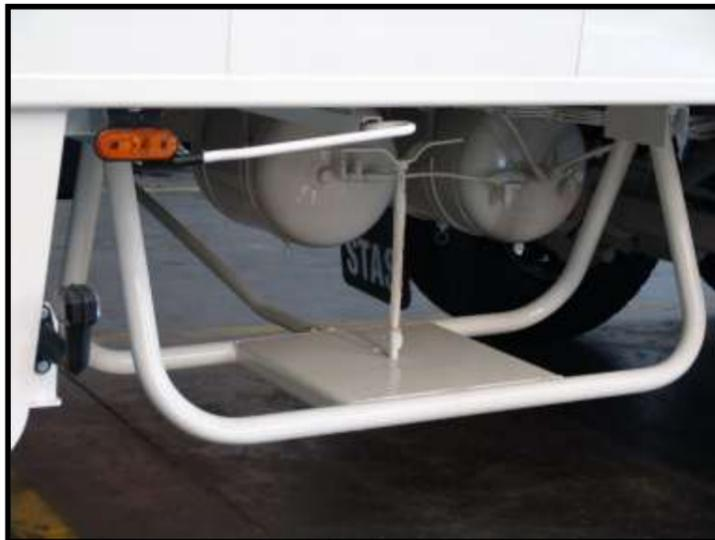
Figure 5.2.a. – Single spare wheel carrier
