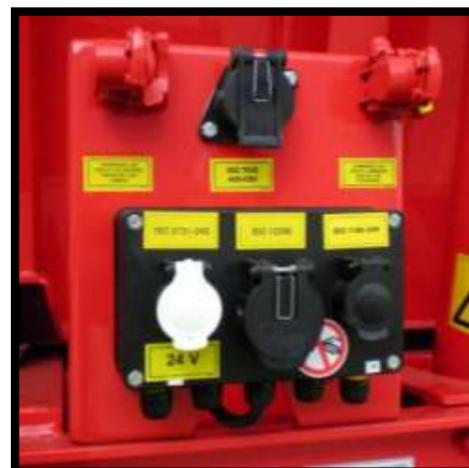
Figure 3.3.a. – Brake system connection
