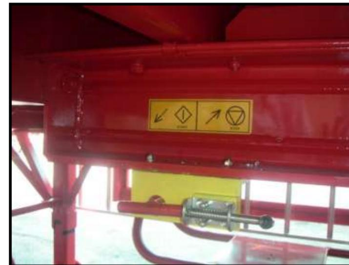
Figure 2.2.4.a. – Mechanical emergency lever in locked position
