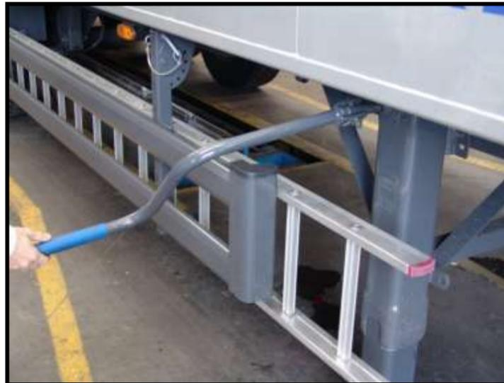
Fig 2.2.1.c. – Handle “steel type” landing leg
