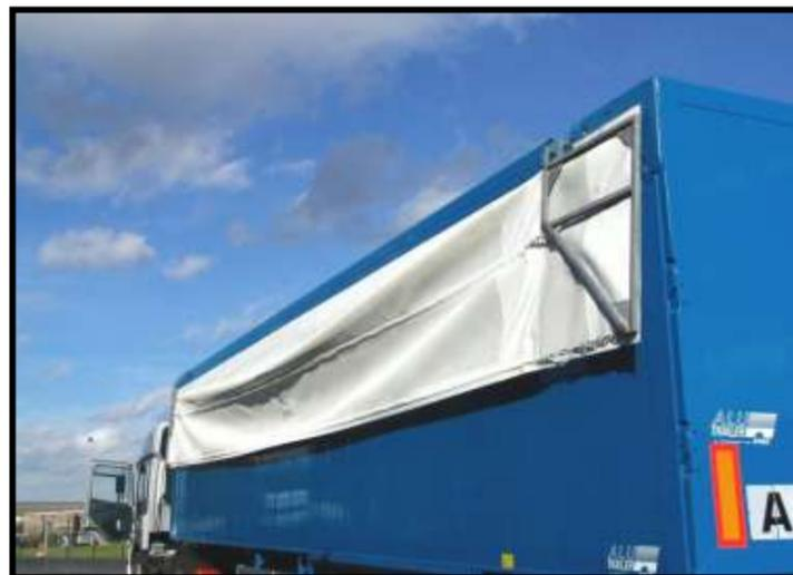
Figure 7.3.a. – Opened left hand section of roof net
