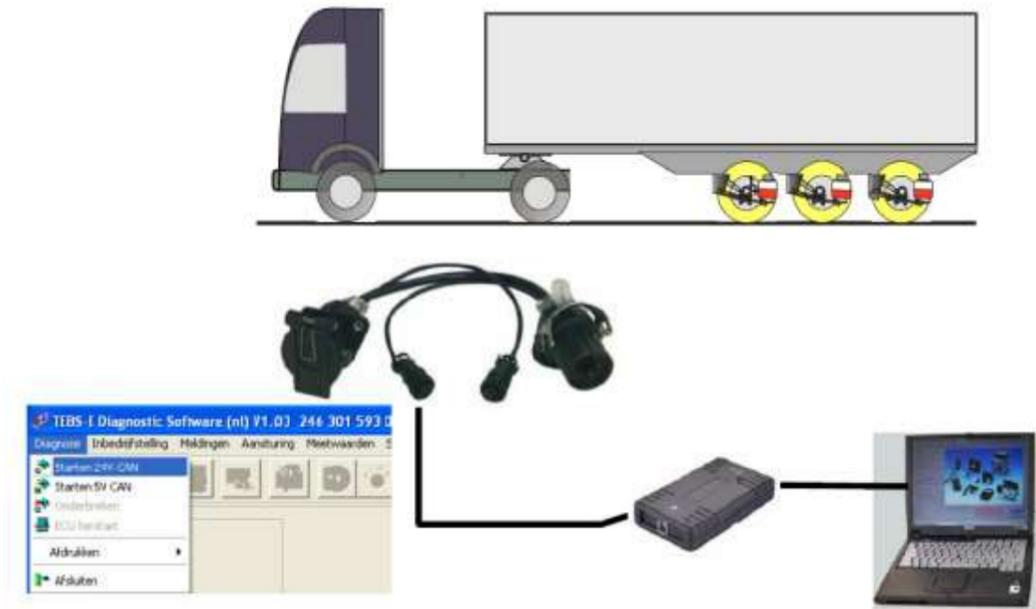
Figure 3.1. – Via Interface and PC with voltage supply ISO7638
