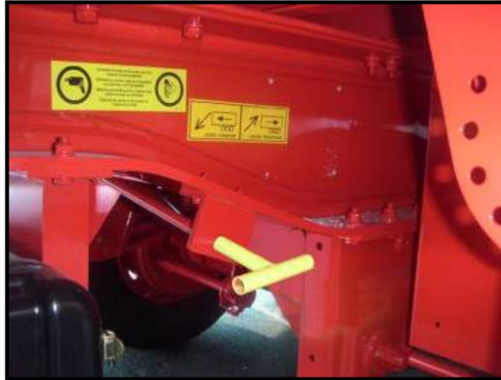
Figure 2.3.3.b. – Selection bar for loading and unloading in unloading position
