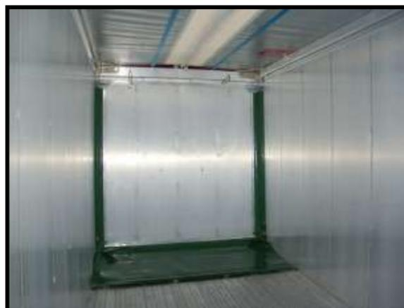
Figure 8.1.a. – Moving bulkhead with floor sheet
