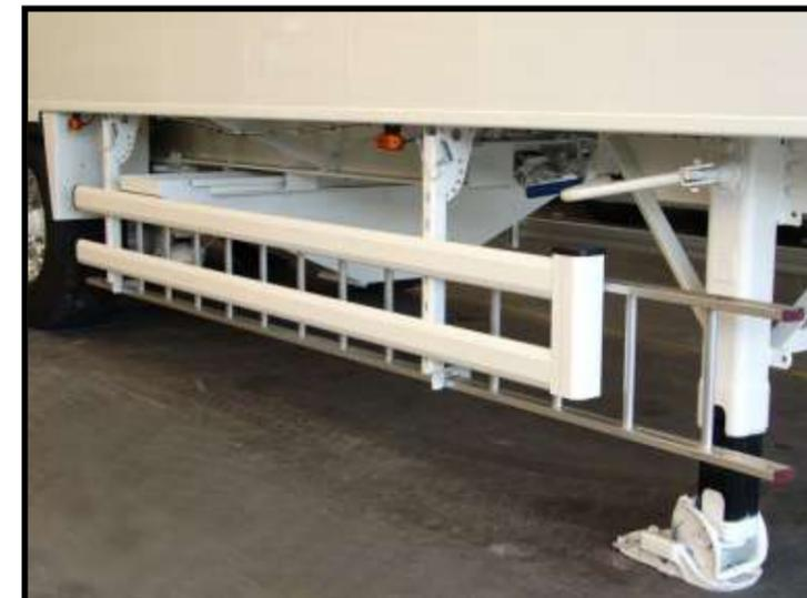
Figure 10.3.b. – Right hand side guard (left for "UK trailer")
