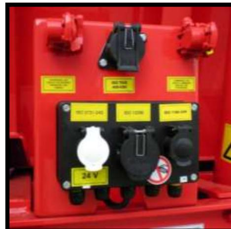
Figure 3.3.a. – Brake system connection
