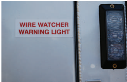
Fig 10 - Wire Watcher Warning Light Located on toolbox - (Located on Off Side of Vehicle)
