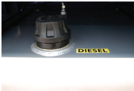
Fig 18 - Diesel Tank (Located Near Side of Vehicle)
