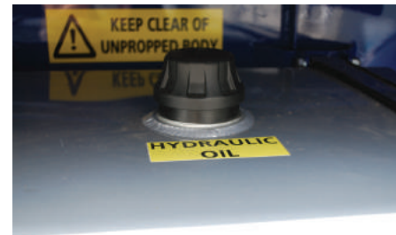
Fig 19 - Hydraulic Oil Tank (Located Near Side of Vehicle)
