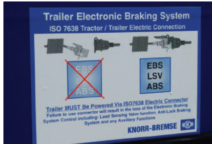
Fig 11 - Trailer Electronic Braking System - Warning Trailer must be powered via ISO7638 Electric Connector (Located on front of trailer)
