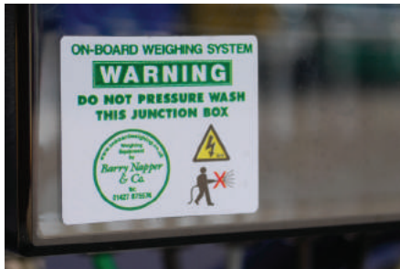
Fig 4 - Do not pressure wash this junction box (On Board Weighing System) (Located in centre front of chassis and on Weigher Control Panel - Vehicle Off Side)
