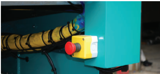
Emergency Stop Switch - Immediately stop all operations
