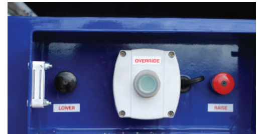
Tipping Control Type C FR-1 Located at front of trailer
