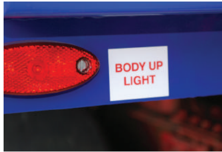
Fig 8 - Body Up Light Warns when vehicle is tipped (Located at front of vehicle)
