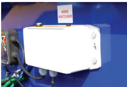
Fig 21 - Wire Watcher Control Box (Located Near Side of Vehicle Inner Chassis)
