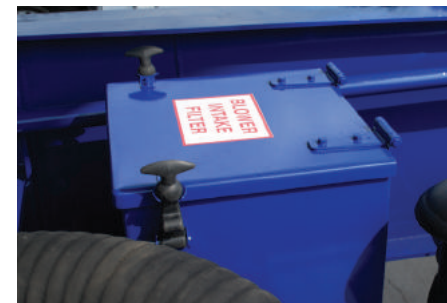
Fig 22 - Blower Intake Filter (Located Centre of Vehicle Chassis)
