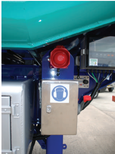
Deep Sea Electronic Unit - Engine Start Up and throttle control
