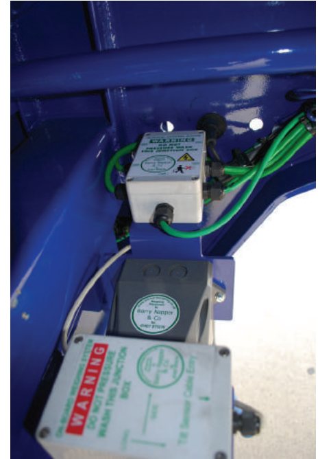
Control Unit - On Board Weigher
