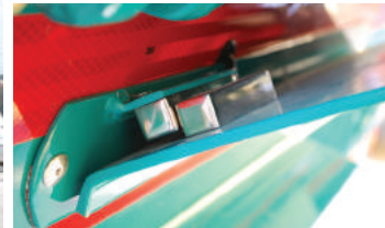
Coded Safety Cut Off for hydraulic functions
