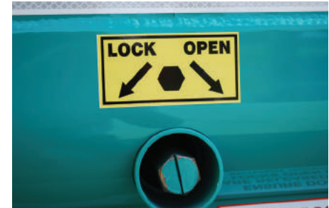
Fig 16 - Internal Doors Open | Close Mechanism (Located Off Side of Vehicle)
