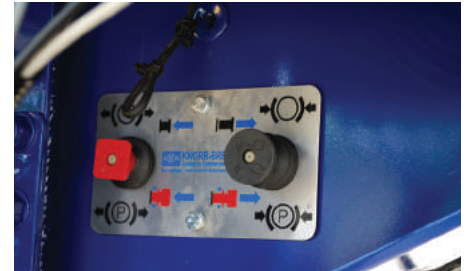
Park Shunt Valve | Parking Brake
