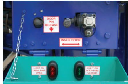
Fig 15 - Muldoon Auto Door Control Panel (Located Off Side of Vehicle)
