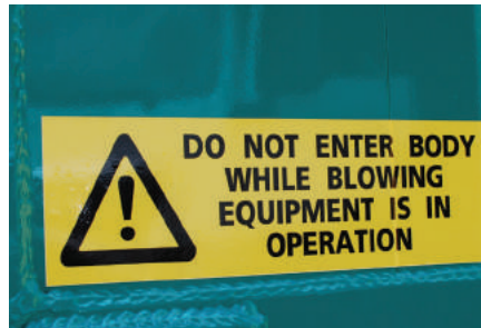
Fig 5 - Do not enter body while blowing equipment is in operation (Located on rear door of trailer)
