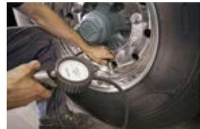
The correct tyre pressure prevents unnecessary tyre wear and reduces the chance of a blow-out. You also save money on fuel costs by maintaining the correct tyre pressure.
