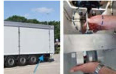
Due to frequent use and pollution, the pneumatic rear door locking device may no longer function optimally. In this case, clean the locking mechanism and immediately lubricate the pneumatic rear door locking device. This to prevent unsafe situations. There are two lubrication points at the bottom of your trailer. Clean the lubrication points and then lubricate them with a grease gun.
