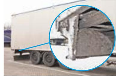
Each light cover contains a sealing rubber to protect against moisture and pollution. A proper seal is crucial for the life of your lighting system.
