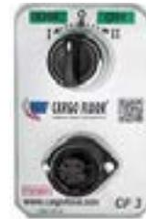
To prevent an operation conflicting with the CF4 remote control, the switch is equipped with an automatic spring return. Position I and II, always jumps back to the "0" position. At the front of the CF3 switch is a connector to which the CF4 switch can be connected. The CF3 switch can be used if the CF4 switch malfunctions
