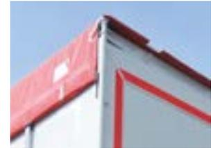
Head load increases the wear pattern of the roof sheet. After departure, the load will settle, causing the straps to loosen. Check the lashing straps en route and keep them tight
