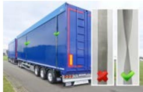
When tensioning the straps, they will rub against the side wall and bottom edge. Protective parts in good condition are therefore required. To prevent paint damage, replace worn protective parts immediately.
