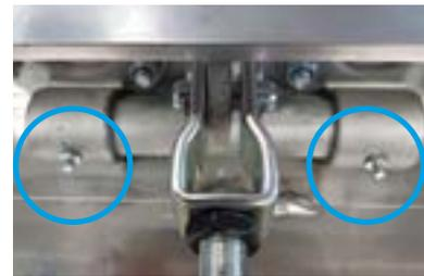
Lubricate with a grease gun.
