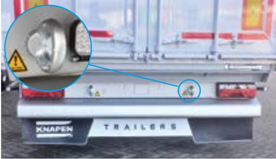
The towing eye can be mounted on one or two sides (load: max. 3 tonnes)
