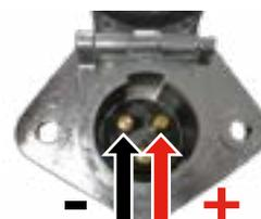
Use the spiral cable supplied with the trailer to power the system. Always check before use that the locking device is in place.
