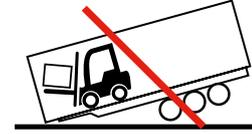
The moving floor must be in the rearmost position.
