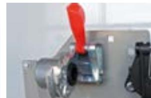
Hang up the air lines again after uncoupling. This prevents sand/pollution in the air connections, which can enter the EBS modulator through the compressed air.
