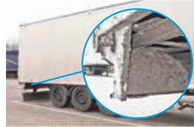
Each light cover contains a sealing rubber to protect against moisture and dirt. A proper seal is crucial for the life of your lighting system.
