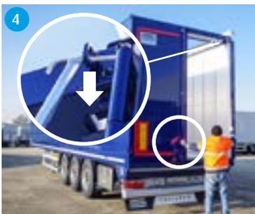
4 Use the sheet stick to pull down the locking devices on the upper beam. Pull open the left rear door at the same time.
