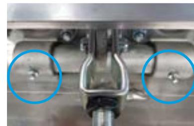
Lubricate with a grease gun.
