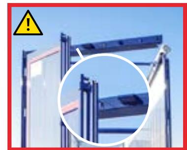
**Only release the upper beam when the cam lock is in the second position as described in step 3.**
