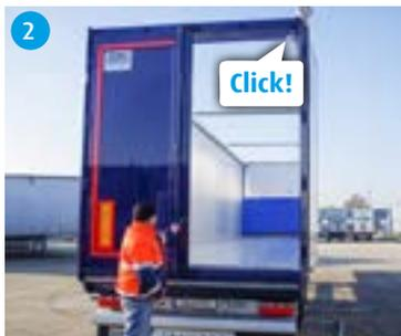
2 Swing the upper beam back into its locking device.
