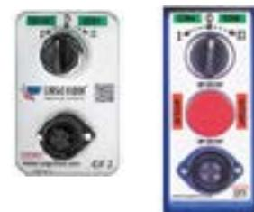
To prevent an operation conflicting with the CF4 remote control, the switch is equipped with an automatic spring return. Position I and II, always jumps back to the "0" position. At the front of the CF3 switch is a connector to which the CF4 switch can be connected. The CF3 switch can be used if the CF4 switch malfunctions.
