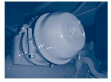
Figure 3.9.a. - spring brake cylinders
