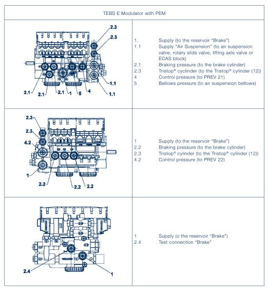
Figure 3.2.2.a. - Pneumatic connection
