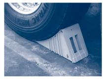
Figure 5.3.a. - Wheel chock in holder (left) and in place (right)
