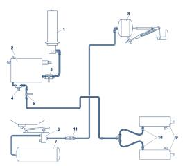
Figure 6.5.1.b. - Diagram Tipper with hydraulic top hinged door
