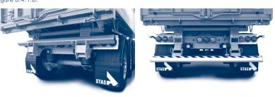
Figure 8.4.1.b. - Automatic hinged rear under-run bar
