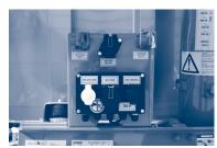
Figure 3.3.a. - Connection braking system
