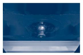
Figure 1.a. - Fifth wheel rubbing plate with kingpin
