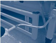
Figure 2.2.1.c. - Landing leg handle "steel type
