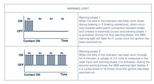
The warning is interrupted when the trailer exceeds a speed of 7 km/hour. In case of system faults, the ABS warning light is permanently activated.
