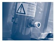
Figure 4.1.a. - Cylinder type plate + maximum cylinder pressure pictogram
