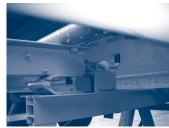
Figure 10.3.c. - Side guards folded up and secured
