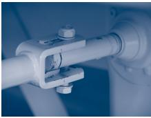
Figure 2.2.1.b. - Landing leg handle "steel type" pulled out
