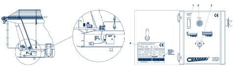
Figure 7.4.2.a. - Electrically operated roof sheet, type "Cramaro"
