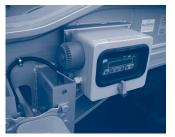
Figure 8.5.1.a. - Weighing equipment measuring unit
