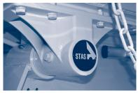
Figure 3.a. – Bolts for tipping shaft locking
