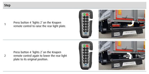
Before taking part in traffic, always check that the folding rear light plate is in its original, lowered position. Any cargo residues, for example, may prevent the rear light plate from lowering completely.
