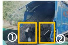
**Important:** Before closing the rear panel, check whether any objects have become wedged on the centring plates.
