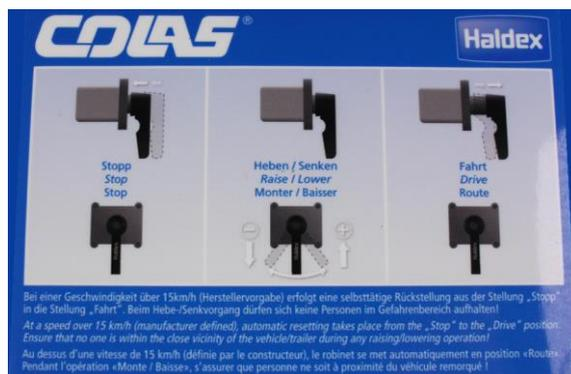
Fig. 29: Raising and lowering with air suspension
