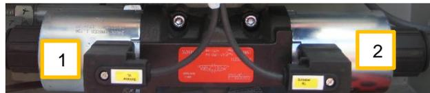
Fig. 45: Slider control valve
