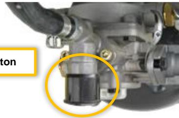
"Release" operating mode for moving the uncoupled trailer is triggered via the trailer release valve.
