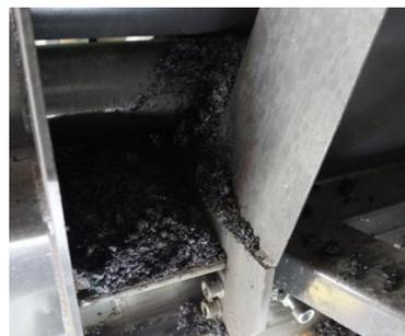
Fig. 66: Asphalt deposits on the slide rail
