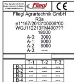
Type plate to specifically identify the machine.
