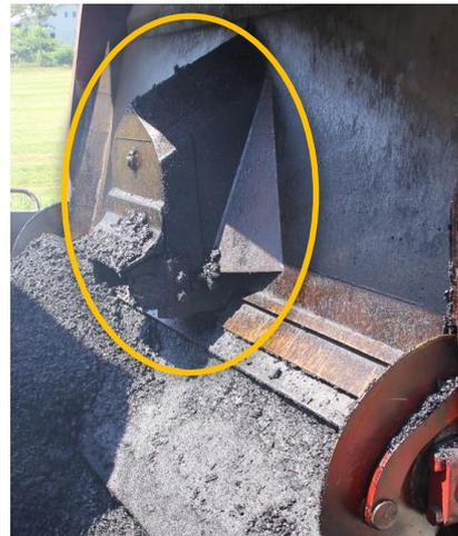
Fig. 58: Closing the rear panel
