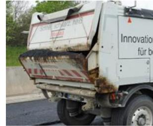
Fig. 60: Partial unloading
