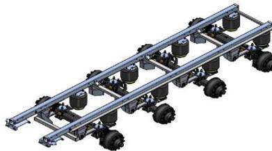
Fig. 106: Four-axle air suspension
