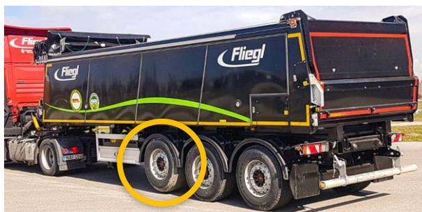
Fig. 77: Lift axle
