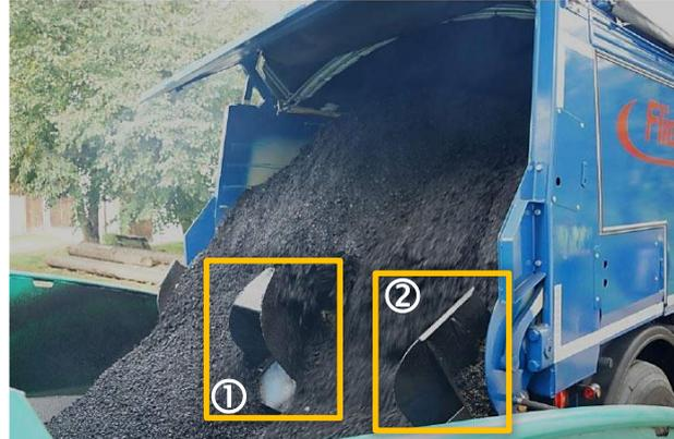
Fig. 64: Discharge chute and centring plates
