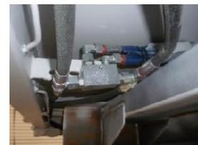
Fig. 4: Shut-off valve
