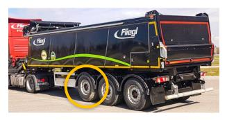
Fig. 77: Lift axle
