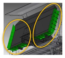
Fig. 94: Checking the moving panel strips on the moving panel and sliding floor
