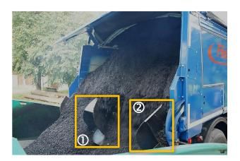
Fig. 64: Discharge chute and centring plates
