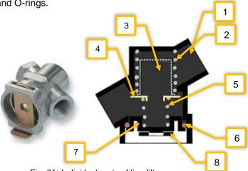
Fig. 91: Individual parts of line filter
