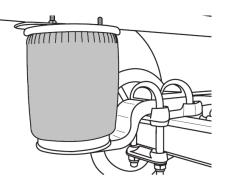
Fig. 93: Air suspension
