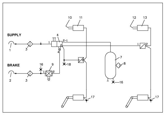
Fig. 101: Compressed air diagram with mech. ALB
