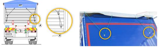
Fig. 110: Attachment of rear straps
